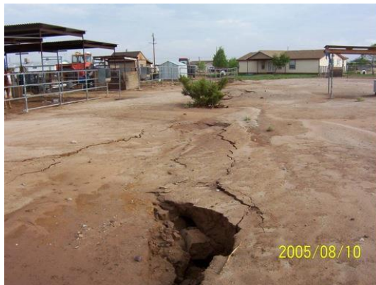
Earth fissure identified during trenching near an earth dam.
